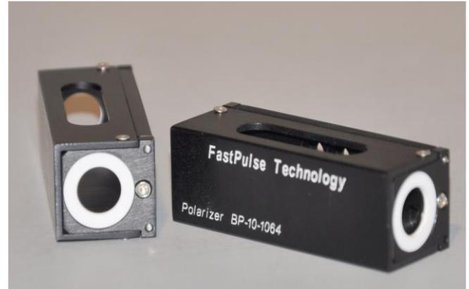
Plate polarizers with coatings provide very high extinction from single and double plate designs. BP Series standard polarizers incorporate 2 plates angled at  $65^\circ$  and mounted in a "V" orientation so there is no beam offset. Precision mounting methods insure stress free high performance.
